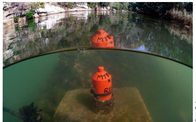
An acoustic receiver deployed in the Mtentu Estuary to monitor the movements of giant kingfish entering this estuary during the summer.
