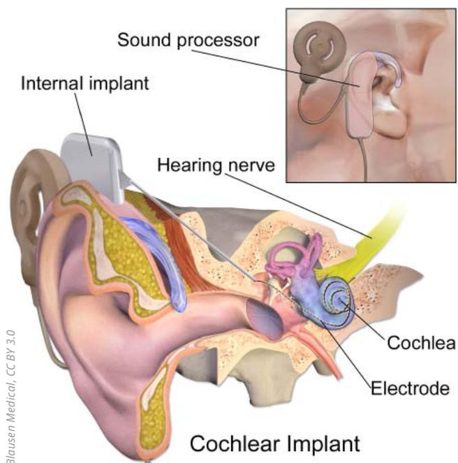
A cochlear implant works as follows. The external sound processor picks up sounds and converts them into digital information, which is then transferred through the coil to the internal implant. The implant converts the digital information into electrical signals and sends these down to the electrode array in the cochlea. The electrode array stimulates the hearing nerve, which sends information to the brain.
